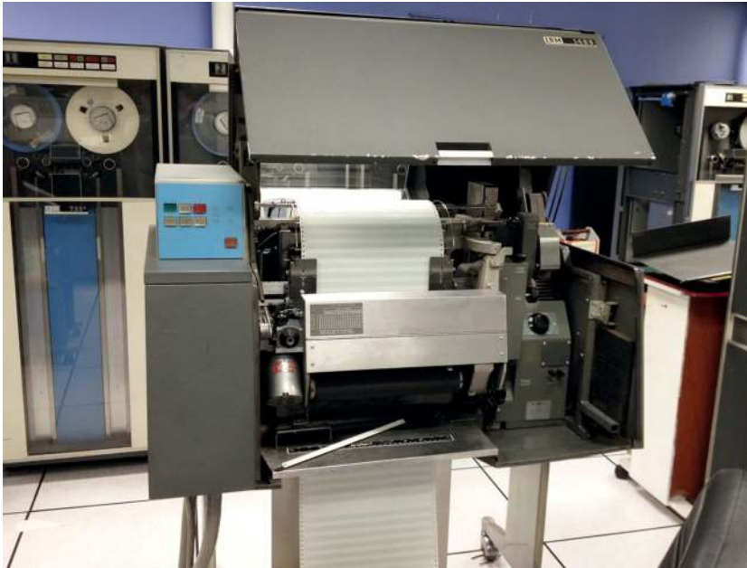
Figure 1.4: The IBM 1401 of the early 1960s incorporated tape drives as storage media for sequential processing.
